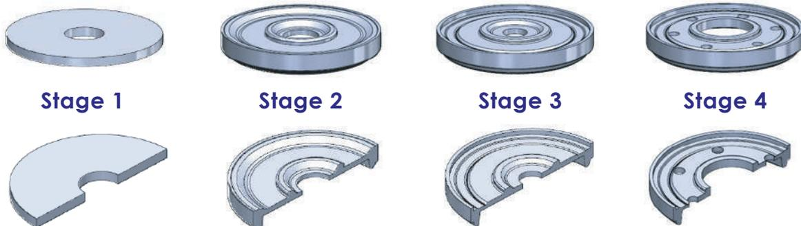
Above is a simplified illustration of operations performed in cold forging of a hard disk clamp:
