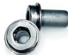
Compared to cold heading, machining produces 4.2g more scrap, which is enough material to cold form a second piece. Besides, the presence of dies ensures high repeatability, and allows for cold heading rate that is in excess of 100 parts-per-minute versus the long cycle time of machining.
